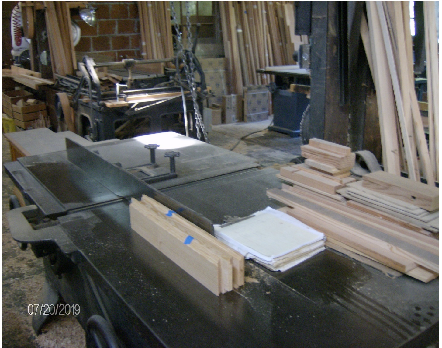
A 36" wide jointer for smoothing lumber
