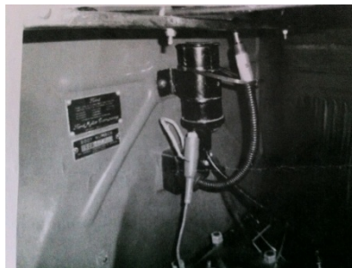
The by-pass cable is installed in the spare distributor and clipped to one side of the coil where the red wire was removed.
