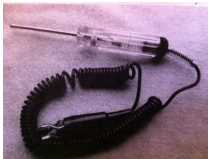
A trouble light can be purchased at any auto parts store. They work on both 6-volts and 12-volts
