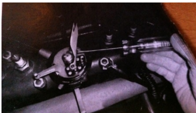
With a piece of paper between the ignition points, and the key turned on, the trouble light should light indicating battery voltage is reaching the points.
