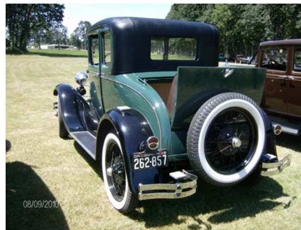
The 1928 Special Coupe. Note leather trim on back of top down to beltline
